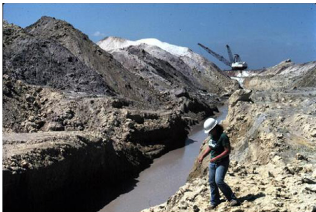
Fig. 1. Dragline mining of phosphate ore in Florida.
