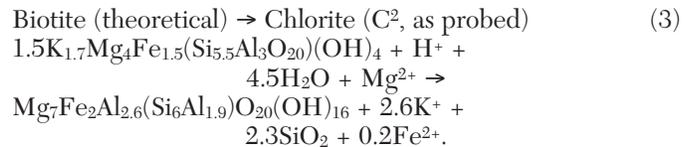
Only water, magnesium, and hydrogen were needed for this reaction to proceed, liberating potassium, silica, and some iron, which would have been added to the fluid. Minor chloritization of hornblende also occurred at this stage. These two reactions were followed by the chloritization of illite in the ore zone:
